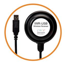
The IWR-USB Gateway provides a link between wireless sensors and any PC with a USB connection.
