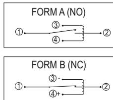
NOTE: COIL POLARITY IS IMPORTANT FOR FORM B VARIANT ONLY.
