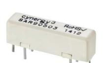
The S series relay was developed for the high voltage ATE market, where printed circuit board space is at a premium. The S series high voltage relay offers a 3kV or 5kV\* isolation performance in a 30mm package.
