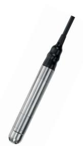
The ILTS is designed for use in continuous submersion in liquids such as water, oil and fuels. The probe uses the latest piezoresistive media-isolated silicon sensing technology and a stainless steel diaphragm. Housed within a 316L stainless steel, or high grade Duplex stainless steel housing, this submersible transmitter is the ideal product for hydrostatic level measurement where temperature is also a critical part of
