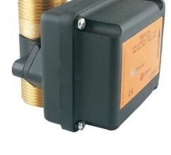
The FSV10AR can be used to control a pump or some other equipment or process via a relay output. If used in a pumped system, the device has to be fitted in the pipe above the pump.
