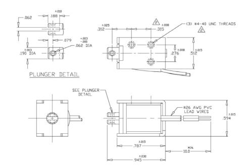
Solenoid shown energized with plunger fully seated
