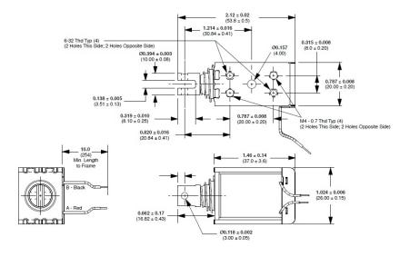
See website for coil connection and operation details Solenoid shown latched with plunger fully seated
