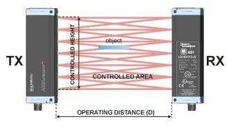
The beam interruption due to the passage of an object inside the controlled area causes the closing of the switching output and the variation of the device analogue output signal. Small objects can be detected (reaching dimensions of only 0.5 mm) and with a reduced surface area.
