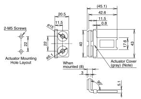
Note: The actuator cover and the actuator stop film are supplied with the actuator and used when adjusting the actuator position.
