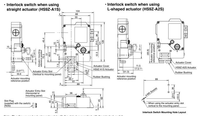
Note: Plug the unused actuator entry slot with the slot plug supplied with the interlock switch.
