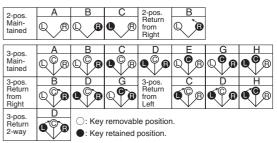
Color Code (except for selector and key selector switches) Illuminated Pushbutton and Pilot Light:
