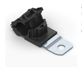
Ratchet P-Clamp, 0.50 - 0.77" Bundle Dia, 180° Short, 0.41" Hole Dia, PA66HIRHSUV/ST/ZN, Black, 20/bag
