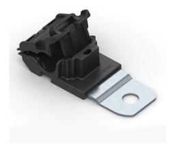
Ratchet P-Clamp, 0.24 - 0.54" Bundle Dia, 180° Short, 0.26" Hole Dia, PA66HIRHSUV/ST/ZN, Black, 5/bg
