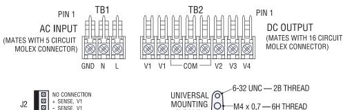
INPUT & OUTPUT CONNECTIONS: 6-32 SCREW WIRE CLAMPS ON 0.312" (7.9mm) CENTERS. 0.045" (1.1mm) SQUARE PINS ON 0.156" (3.96mm) CENTERS;
