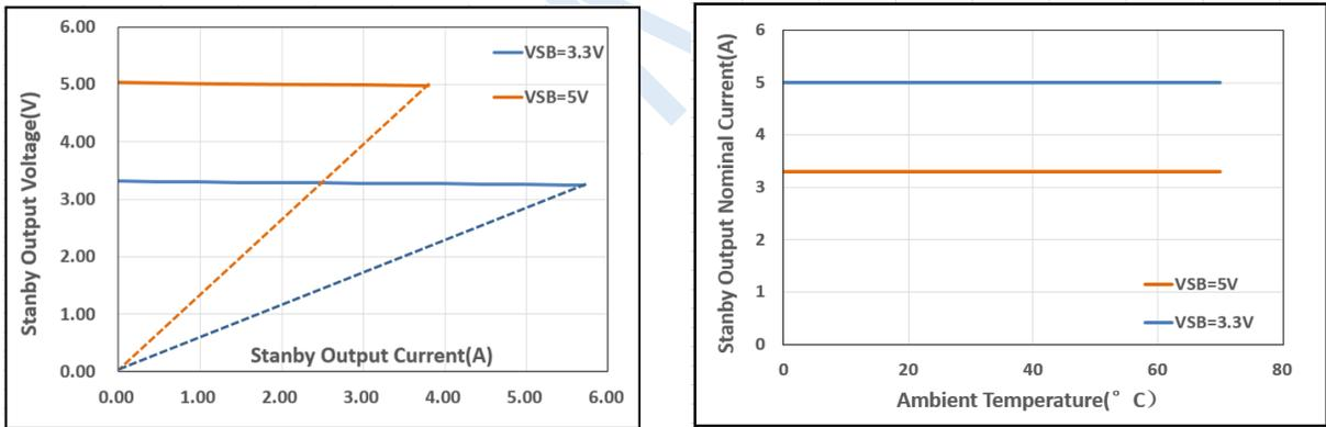
Figure 7. Current Limitation and Temperature Derating on 3.3 / 5 V<sub>SB</sub>
