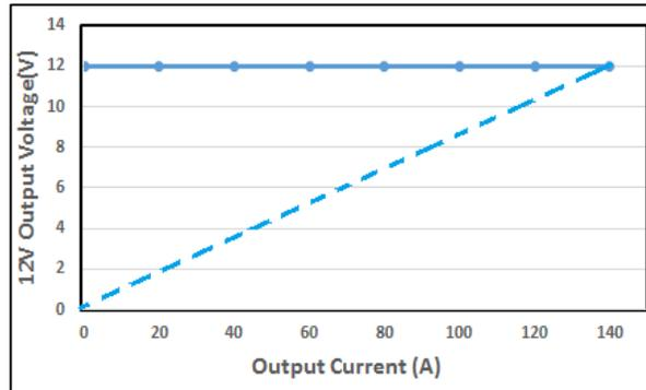
Figure 6. Current Limitation on V<sub>1</sub> (V<sub>i</sub> = 230 VAC)
