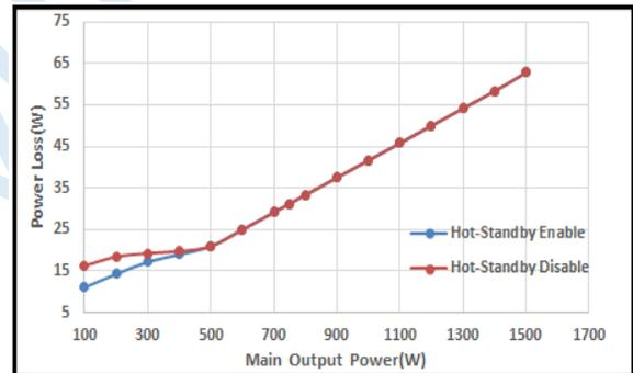
Figure 12. PSU power losses with/without hot-standby mode
