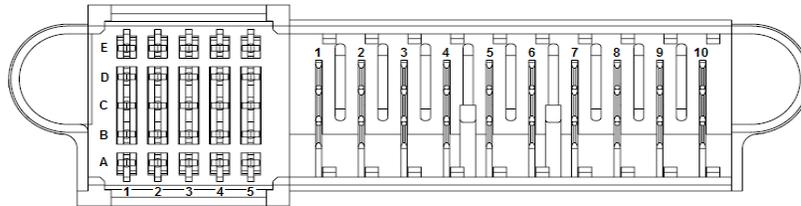
Power Supply Connector: Tyco Electronics P/N 2-1926736-3 (NOTE: Column 5 is recessed (short pins))
