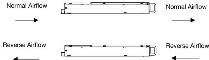
Figure 19. Airflow direction
