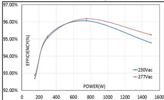
Figure 2. Efficiency vs. Load current (ratio metric loading)
