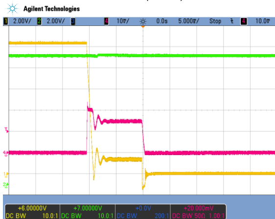
Figure 11. Short circuit on V1 (50ms/div) CH1: V1 (2V/div) CH2: VSB (2V/div) CH4: I1 (200A/div)
