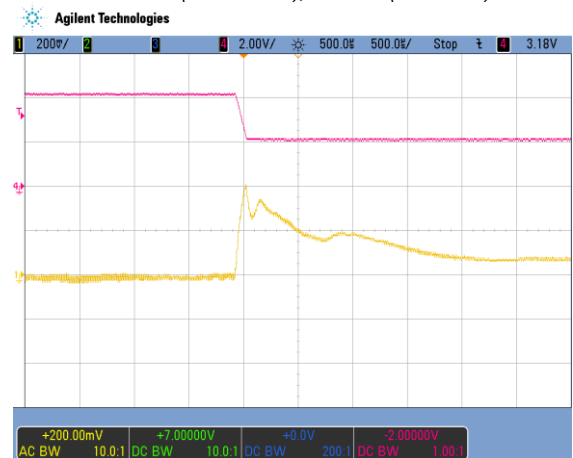
Figure 18 - Load transient V1, 244 to 122 A (500 μs/div) CH1: V1 (200 mV/div); CH4: I1 (100 A/div)
