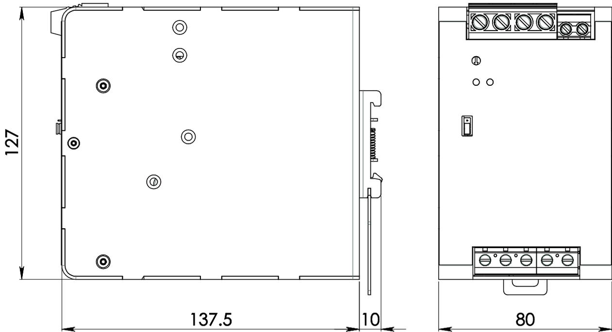
Figure 1. Mechanical Drawing
