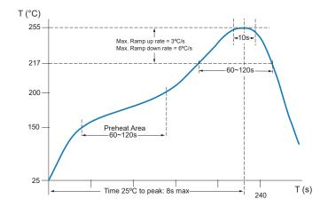
The recommended reflow conditions are set according to the soldering equipment used. Since various manufactures may have different reflow soldering equipment, products, process conditions, set methods, etc., when setting the reflow contions, please adjust and confirm according to users' environment/equipment.
