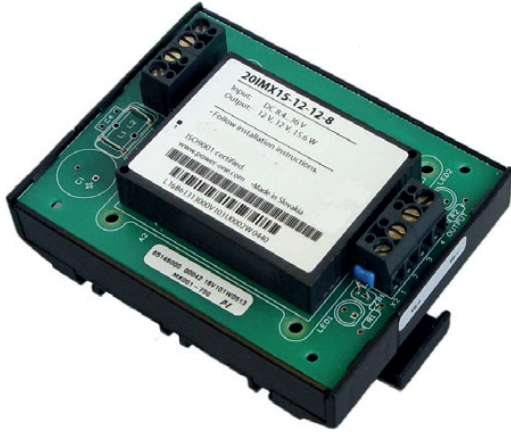
Fig. 24 DIN-rail mounting support HZZ00628-G (previously DMBIMX15)
