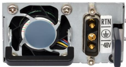
Figure 7. Input polarity marking
