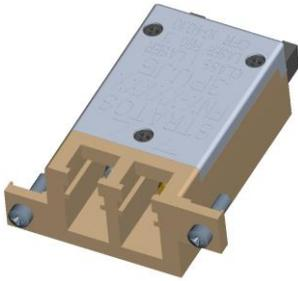
This transceiver consist of transmitter and receiver functions combined in a Low Profile RJ module. The optical transmitter is a high output 1310 nm FP laser. The transmitter input lines are driven with differential LVPECL signals applied to the Transmit (TX+ and TX-) pins. These signals are internally converted to a suitable modulation current by a CMOS integrated circuit. The optical transmitter can be disabled by applying an LVTTTL signal to the Transmit Disable (TDIS) pin.
