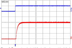
Figure 6. Turn-on transient at full rated load current (resistive) with no output capacitor at Vin = 48 V, triggered via ON/OFF pin.
