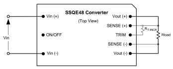
Figure C. Configuration for increasing output voltage.
