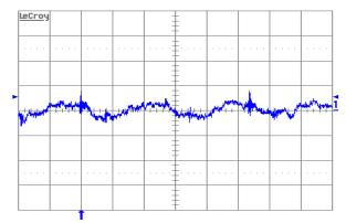
Figure 12. Input reflected-ripple current, is (10 mA/div.), measured through 10µH at the source at full rated load current and Vin = 48V. Refer to Figure 11 for test setup. Time scale: 1µs/div.
