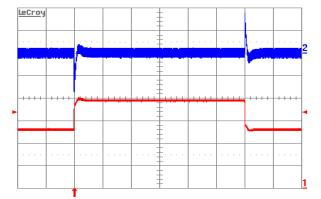
Figure 9. Output voltage response to load current step-change (12.5A–18.75A–12.5A) at Vin=48V. Top trace: output voltage (100 mV/div.). Bottom trace: load current (5A/div.). Current slew rate: 5A/µs. Co=470µF POS+1µF cer. Time scale: 0.2ms/div.
