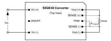
Figure D. Configuration for decreasing output voltage.
