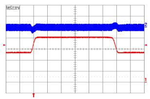
Figure 8. Output voltage response to load current step-change (12.5A–18.75A–12.5A) at Vin = 48V. Top trace: output voltage (100mV/div.). Bottom trace: load current (5A/div.). Current slew rate: 0.1A/µs. Co=1µF cer+10µF tant. Time scale: 0.2ms/div.
