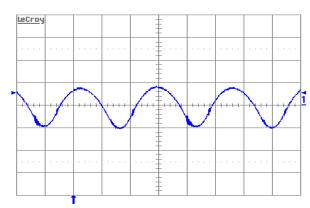
Figure 13. Input reflected ripple-current, ic (200 mA/div.), measured at input terminals at full rated load current and Vin = 48 V. Refer to Figure 11 for test setup. Time scale: 1 µs/div.
