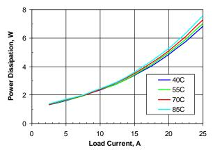
Figure 5. Power dissipation vs. load current and ambient temperature for SSQE48T25015 converter mounted vertically with Vin = 48 V and air flowing from pin 1 to pin 3at a rate of 200 LFM (1.0 m/s).
