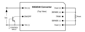
Figure A. Circuit configuration for ON/OFF function.
