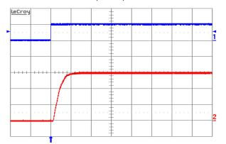
Figure 7. Turn-on transient at full rated load current (resistive) plus 30,000µF at Vin = 48V, triggered via ON/OFF pin. Top trace: ON/OFF signal (5 V/div.). Bottom trace: Output voltage (0.5 V/div.). Time scale: 5 ms/div.
