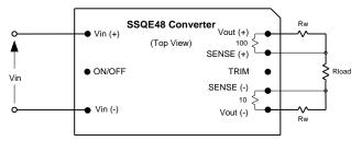
Figure B. Remote sense circuit configuration.
