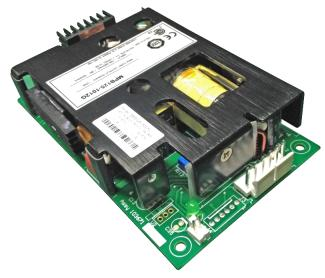
The MPB125 Series incorporates patented high efficiency circuitry, high power density and active Power Factor Correction (PFC) to meet the requirements of networking and data communications systems, as well as commercial and industrial configurations.
