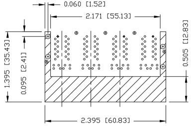
THE SHADED AREA ON THE CUSTOMER BOARD ARE RECOMMENDED TO BE CLEAR OFF ANY VIA HOLE OR COMPONENT PAD.
