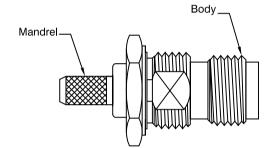
3) Insert the contact into the body and ensure that the contact captivates. Make sure that the braid is on the outside of the mandrel. Slide the ferrule over the braid until the ferrule butts up against the body. Crimp the ferrule using the correct tool for the connector.
