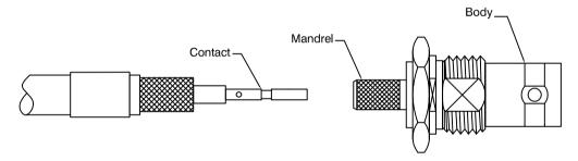
3) Insert the contact into the body and ensure that the contact captivates. Make sure that the braid is on the outside of the mandrel. Slide the ferrule over the braid until the ferrule butts up against the body. Crimp the ferrule using the correct tool for the connector.
