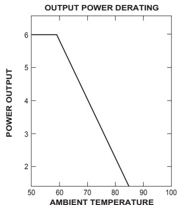
Typical Performance: ( $T_c=25^\circ\text{C}$ ,  $V_{in}=\text{Nom VDC}$ , Rated Load)
