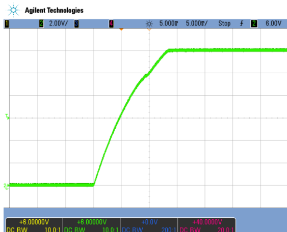
Figure 9 - Turn-On AC Line 230 VAC, full load (5 ms/div) CH2: VSB (2 V/div)
