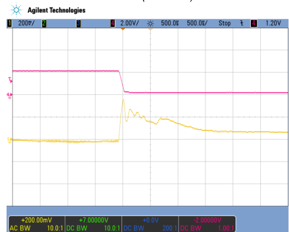
Figure 16 - Load transient V1, 125 to 3 A (500 μs/div) CH1: V1 (200 mV/div); CH4: I1 (100 A/div)
