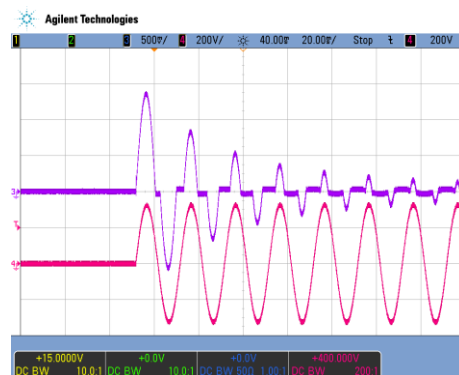
Figure 5 - Inrush current, V_{in} = 230V_{ac} , 0^\circ phase angle CH4: V_{in} (200V/div), CH3: I_{in} (10A/div)
