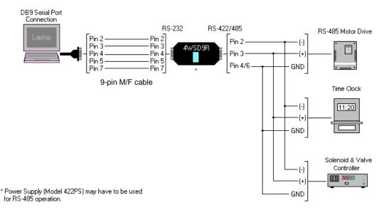
Figure 1: RS-485 2-wire half-duplex diagram
