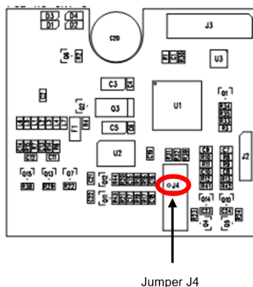
Figure 1: CNT board – setting the binary input current
