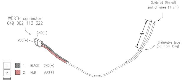
Connector pin-out, view into the router (rear view of cable connector)
