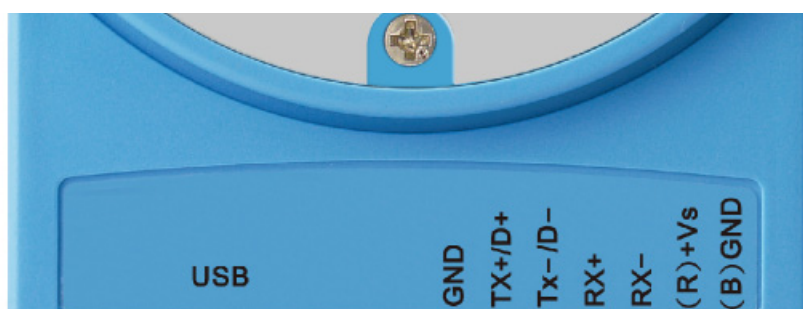
Figure 1.9 RS-422/485 and USB interface of ADAM-2520Z.
