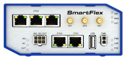
Figure 50: Version with SWITCH board
