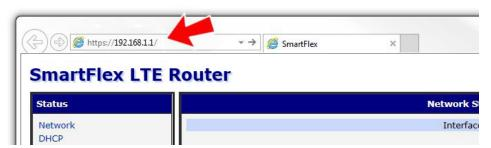
Figure 56: Entering the IP address of the router
