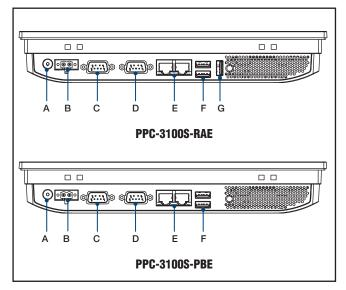
A. Power Switch B. DC-In C. RS-232 D. RS-232/422/485 E. 2 x RJ45 LAN F. 1 x USB 2.0, 1 x USB 3.0 G. USB 2.0
