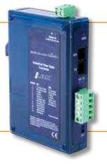
B&B Electronics' ILinx<sup>™</sup> fiber converters designed with functionality required for heavier industrial environments. Model FOSTCDRi-Sx industrial-grade isolated converter changes RS-232, RS-422, or RS-485 to single-mode fiber optics.
