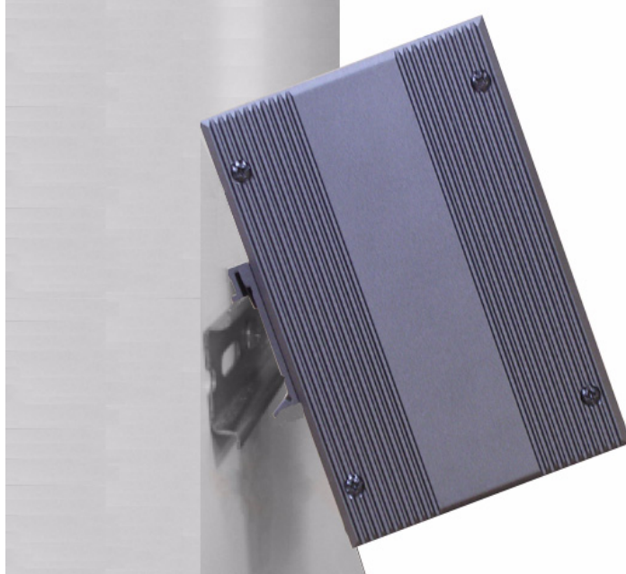
Figure 2.3 DIN-rail Installation Step 1
