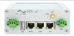
The XR5i v2F industrial router secures connections between two local networks (LAN) via two Ethernet interfaces 10/100. The XR5i v2F can also convert serial RS232, RS485, M-BUS, I/O to IP local area network (LAN Ethernet 10/100). WiFi models are available.
