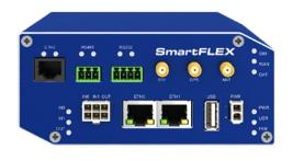
SmartFlex<sup>™</sup> cellular router provides secure Internet connectivity for devices and LANs via the cellular networks. It canprovide automatic wireless failover for wired networks, wireless connectivity for devices in remote locations where cable connections are impractical and wireless connectivity for mobile assets.
