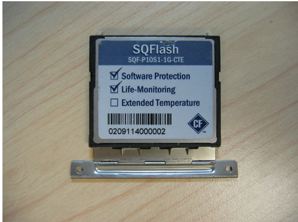
Figure 2.15 Put CF on to the CF tray
