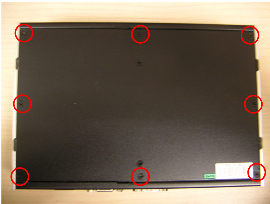
Figure 2.16 Unscrew the screws of bottom cover
