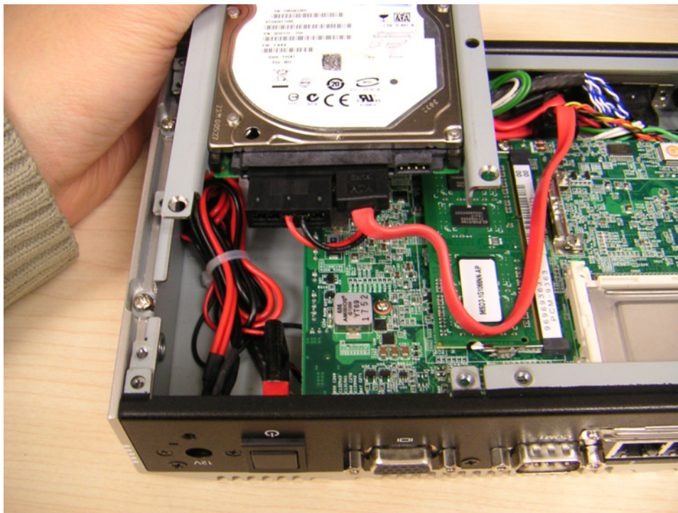
Figure 2.20 Connect the SATA HDD power and signal cables.
