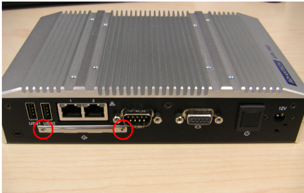
Figure 2.12 Remove the CF door screws
