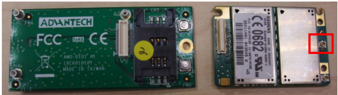
Figure 5.10 AMO-EDGE base board and Siemens module
