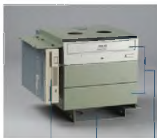
One 3.5" drive bay Three 5.25" drive bays One internal 3.5" drive bay space
