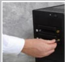
Insert carrier into receiving frame & turn on powered key lock
