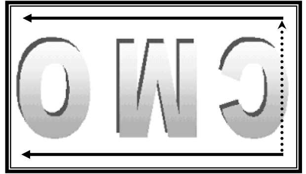
RPFI = high: display with 180degree rotation
