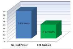
Source: Intel Labs Energy Efficient Ethernet reduces the controller power to approximately 50% of its normal operating level.
