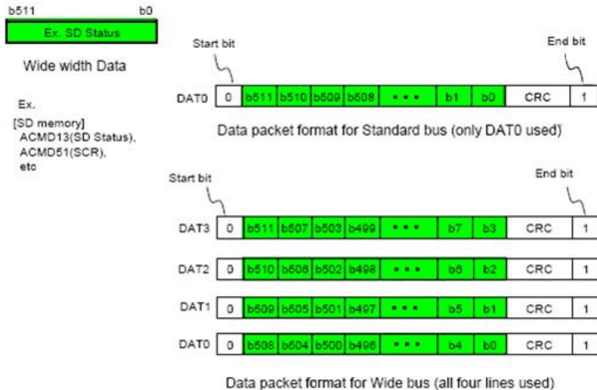
Figure 6-1-7: Data packet format - Wide width data
