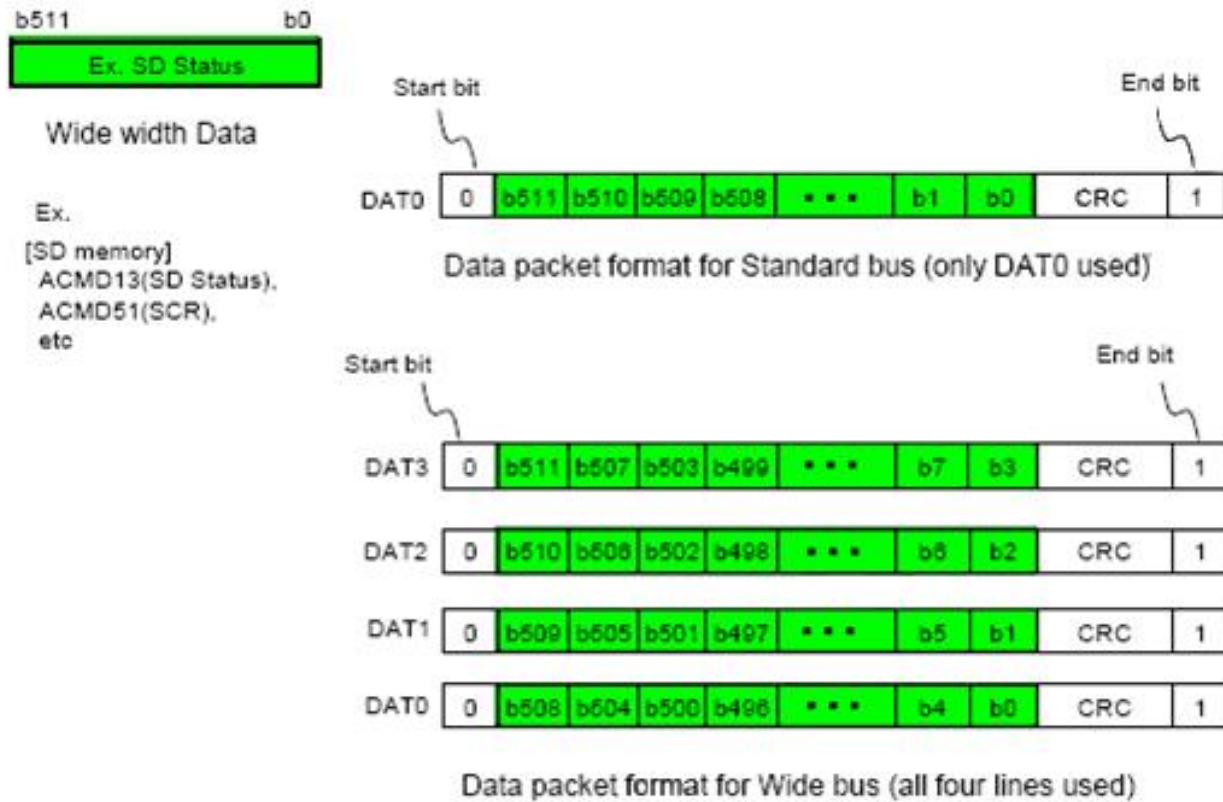
Figure 6-1-7: Data packet format - Wide width data
