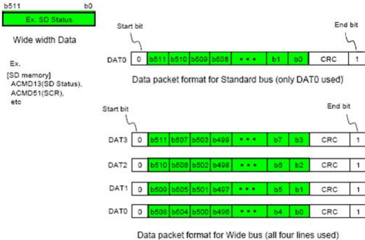
Figure 6-1-7: Data packet format - Wide width data
