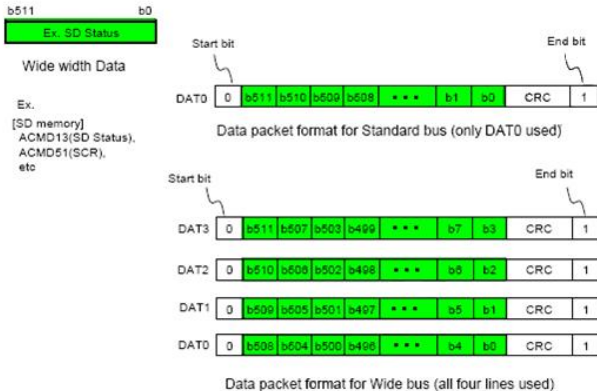
Figure 6-1-7: Data packet format - Wide width data
