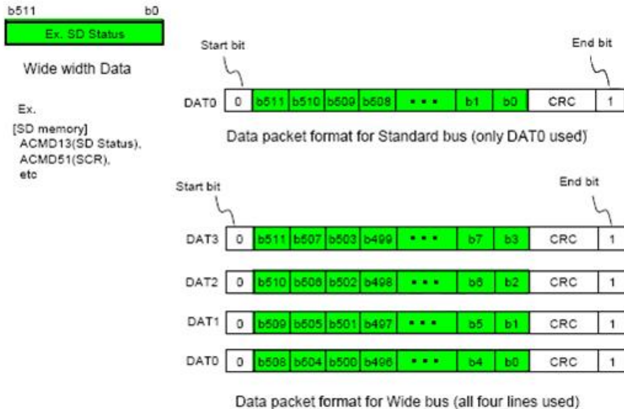
Figure 6-7: Data packet format - Wide width data
