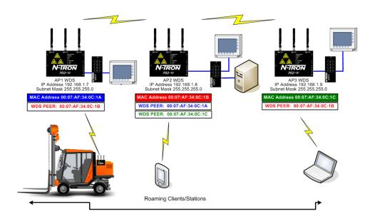
These 702-W wireless radios have been configured as peers. This topology allows forklifts, or other mobile wireless devices, to maintain communication as they move from the area covered by one 702-W into the area covered by the next 702-W.
